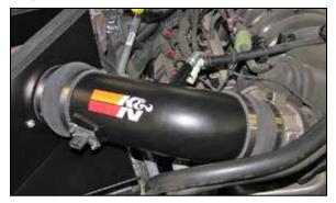
17. Install the K&N<sup>®</sup> intake tube into the hump coupler and then into the step coupler, then adjust the tube for best fit and secure with the provided hose clamps.
