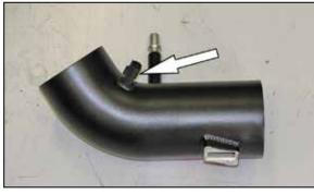
13. Remove the O-ring from the inlet air temperature sensor and then install the sensor into the grommet installed into the K&N<sup>®</sup> intake tube during the previous step.
