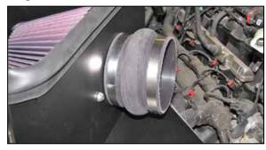
15. Install the provided coupler hump hose (08418) onto filter adapter and secure with the provided hose clamp.
