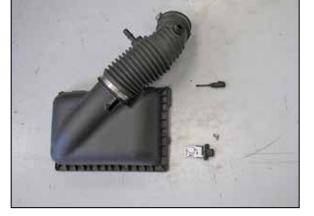
11. Remove the two screws securing the humidity sensor then remove the humidity sensor from the air filter housing. Remove the inlet air temperature sensor from the stock intake tube.
