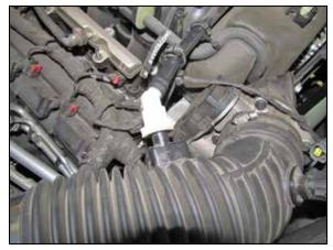
4. Depress the locking tab and then disconnect the crank case vent hose from the factory intake tube.
