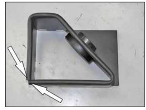
8. Install the provided edge trim onto the  $K\&N^{\circledast}$  heat shield as shown.
