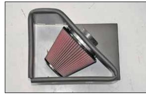
9. Install the K&N<sup>®</sup> air filter onto the filter adapter and secure with the provided hose clamp.
