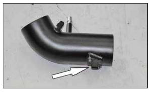
14. Install the humidity sensor into the K&N<sup>@</sup> intake tube and secure with the provided hardware. NOTE: On vehicles not equipped with a humidity sensor, install the provided block off and gasket.
