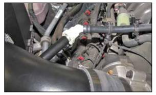
18. Connect the factory crankcase vent hose to the quick disconnect fitting on the K&N<sup>®</sup> intake tube.
