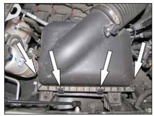
6. Release the four locking tabs securing the air filter housing lid and then remove the housing lid and factory intake tube from the vehicle. Remove the factory air filter.
